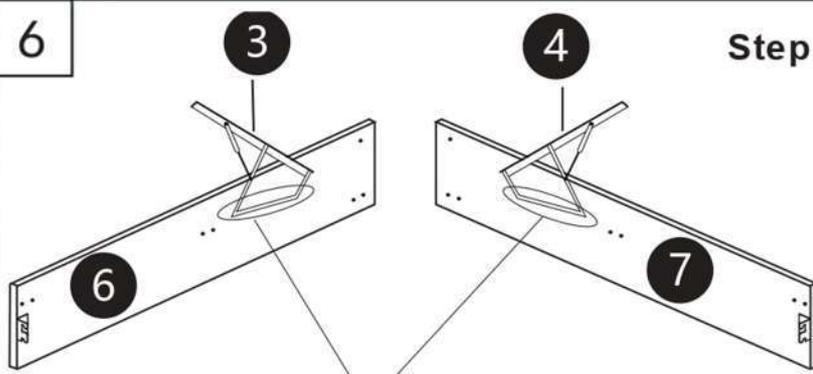
**Step 6: Attach the gas lift mechanism (3 and 4) to the side rails 6 and 7 using hardware N, E and A.**
