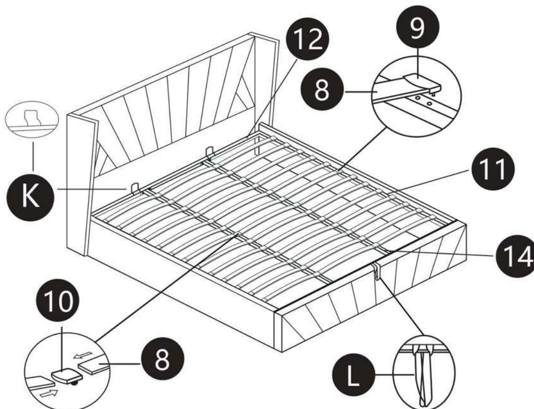
**Step 14(a):** Attach the slats (8) to the plastic clips and insert them into the holes of the metal bars (11 and 14). Clips open from both sides (10) will be attached to the middle bar (14), and clips open from one side (9) will be attached to the side bars (11).
