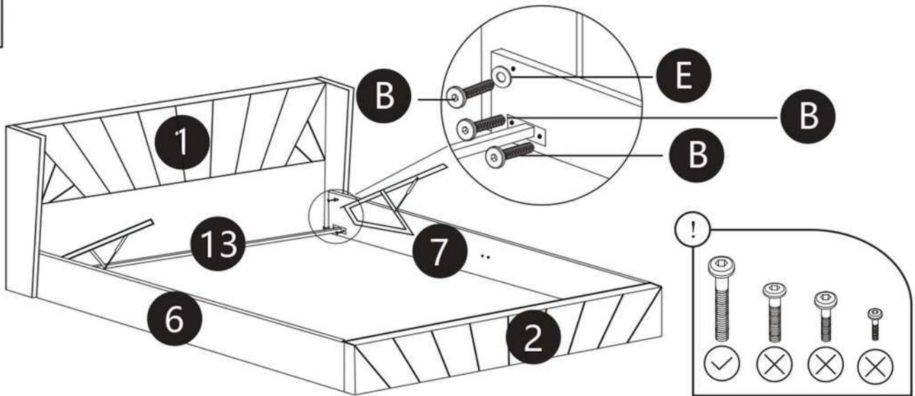
**Step 10: Attach side rail connector (13) to the side rails (6 and 7) and headboard (1) using parts B and E.**
