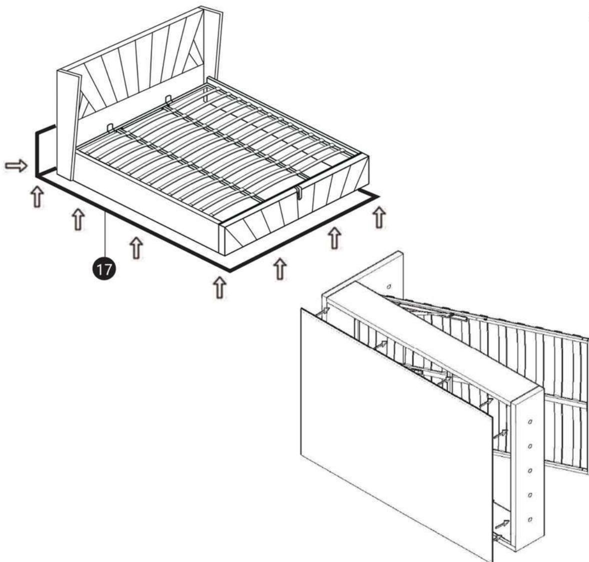
**Step 15 : Attach the non-woven fabric (17) to the back of the headboard.**
